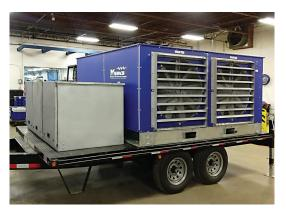
2 MW Trailer Mounted Load Bank
